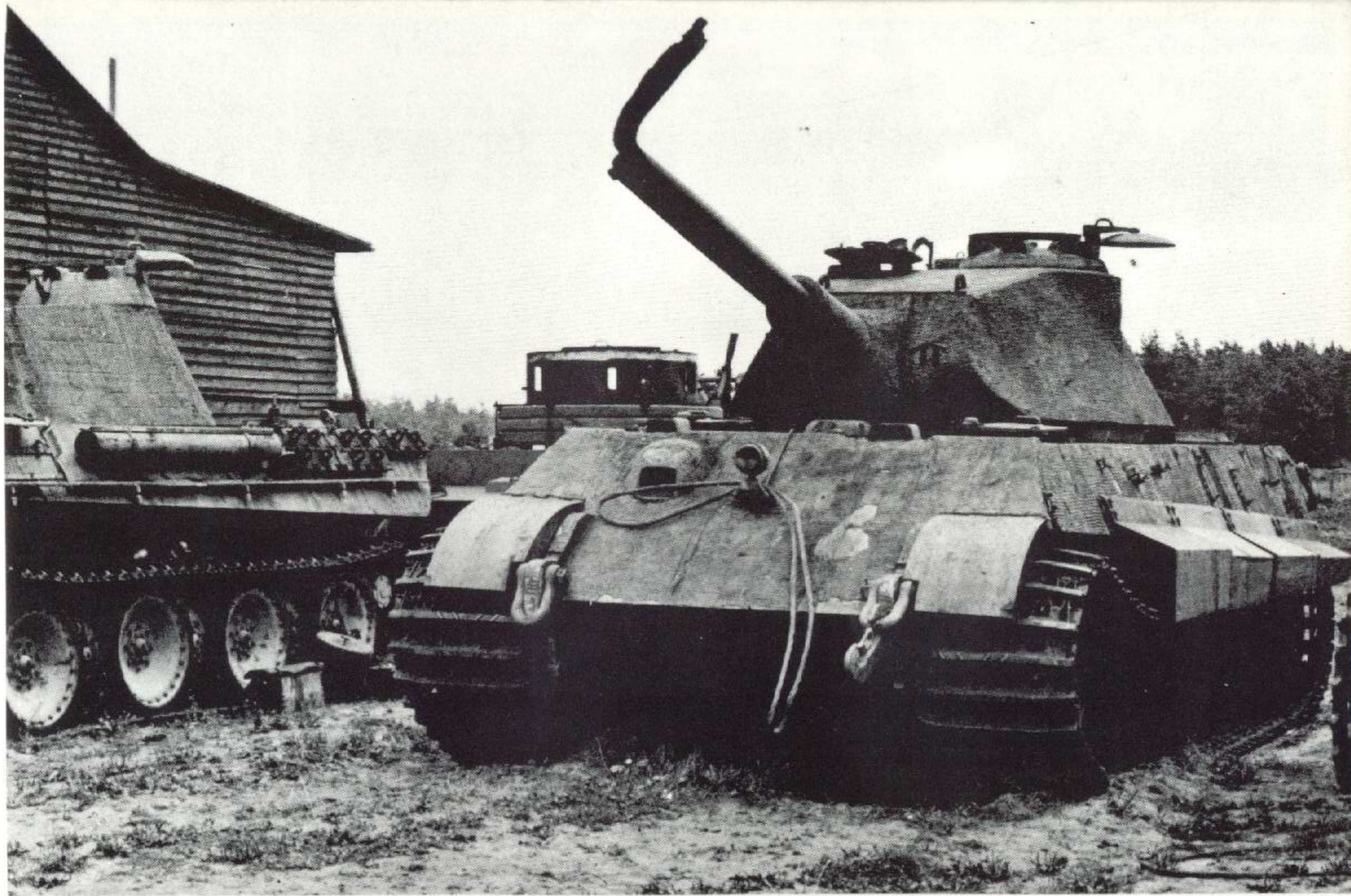
The end: Made useless by barrel damage, this abandoned Tiger (with Porsche turret) waits to be scrapped on the grounds of Tank Unit 500 in Paderborn. To the right of the tank is a Panther V tank, and diagonally behind it the turret weight used on the VK 4501 (H) can be seen.
