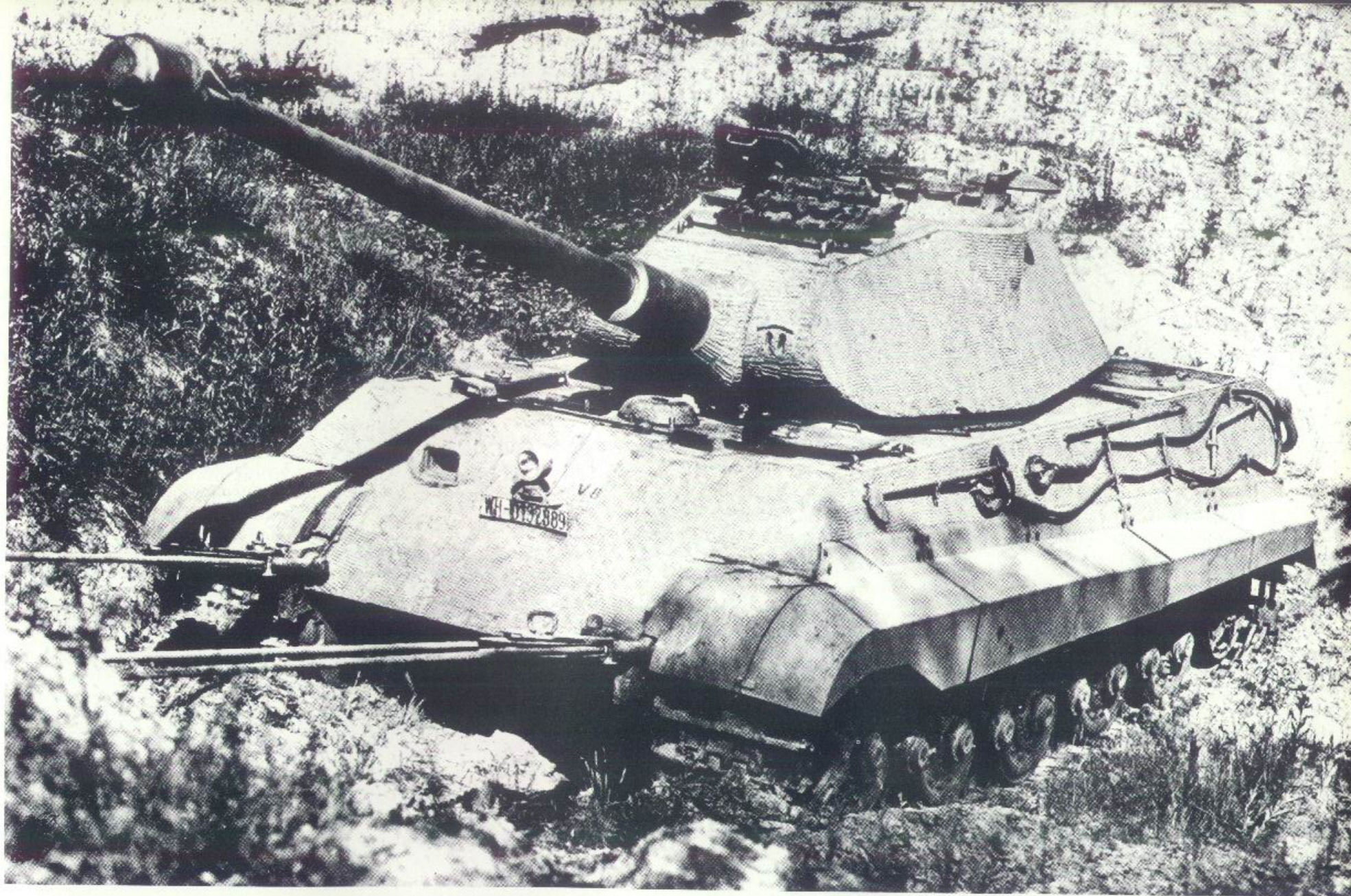
A series of tanks served for testing. This photo shows V8 in a rescue maneuver at Kummersdorf. Notice the number plate — not used in combat — on the bow plate.
