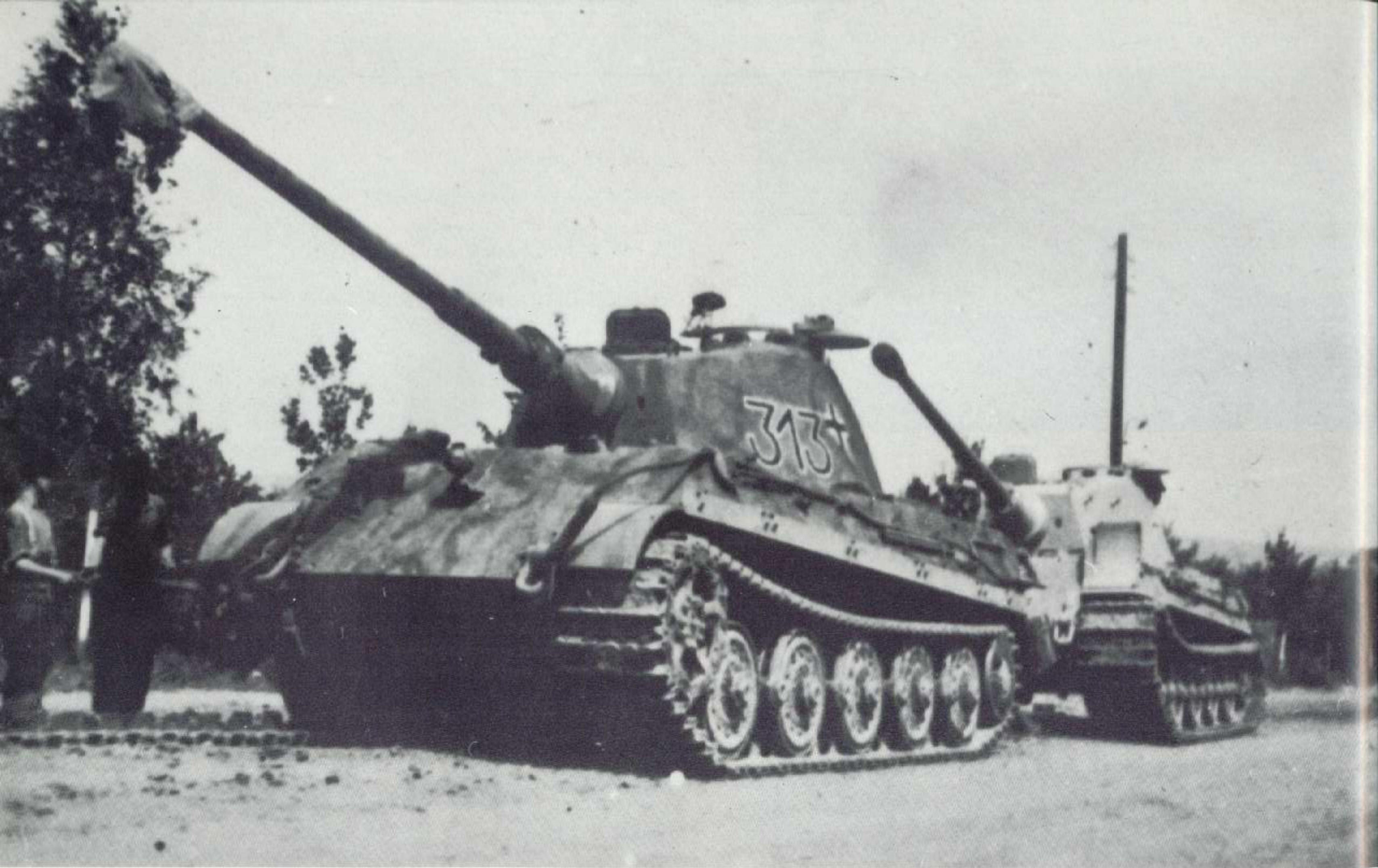
The Heavy Panzer Battalion 501 unloading its tanks at Kielce, Poland. Tank 313 is being pushed by a second Tiger onto the right-side combat track laid out ahead of it. The narrow shipping track is still on the left side. Then the track aprons will be screwed on.
